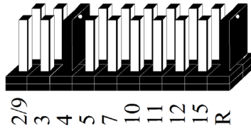
Figure 3 - Header J2, IRQ Selection (Factory Default)
