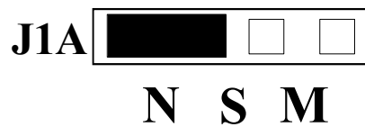
Figure 5 - Header J1A, Normal IRQ Mode
