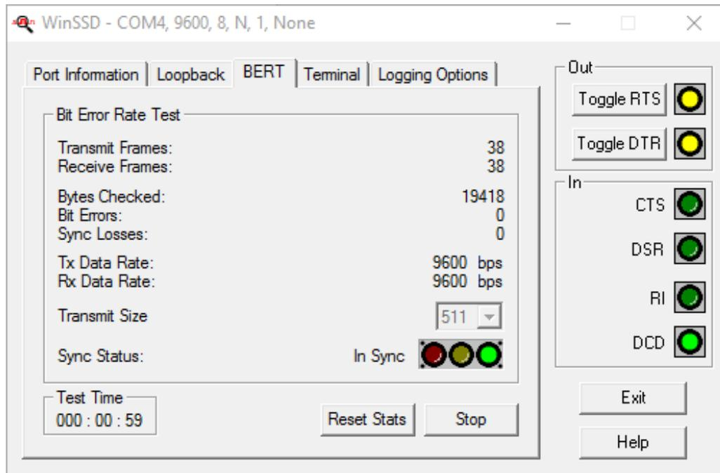
This verifies that the adapter is working properly. You can continue testing this port with different configurations or proceed with testing other ports, if necessary.
