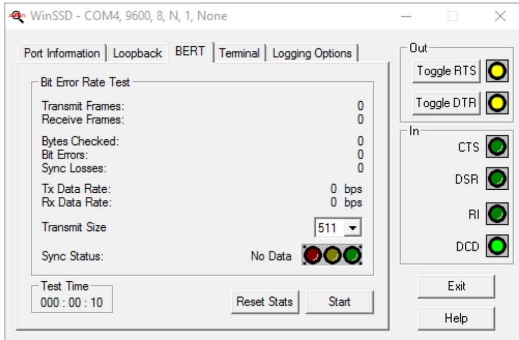
If the COM port is properly working, the Sync Status green light will glow and the Transmit Frames and Receive Frames will increase. The Tx and Rx Data Rates will show the calculated data rate.
