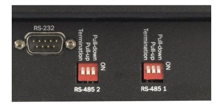
Each RS-485 Isolated port has selectable line conditioning via three DIP switches. These switches control RS-485 line termination and pull-up and pull-down resistors.
