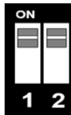
Figure 8: Auto-RS485 is ENABLED and DTR is selected as the RS-485 direction control signal
