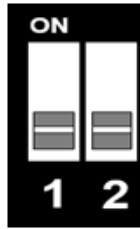
Figure 5: Auto-RS485 is DISABLED and RTS is selected as the RS-485 direction control signal
