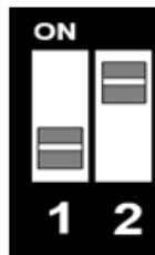
Figure 6: Auto-RS485 is DISABLED and DTR is selected as the RS-485 direction control signal This is the default configuration for SW1 on the 7804c.
