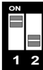
Figure 7: Auto-RS485 is ENABLED and RTS is selected as the RS-485 direction control signal
